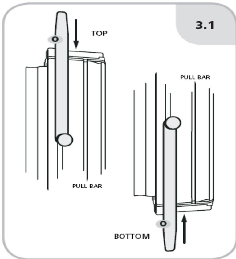
The Slide Bolt locks are installed on surface of the Milano pull-bar that faces inside. It uses the slot that is furthest away from the magnet.
