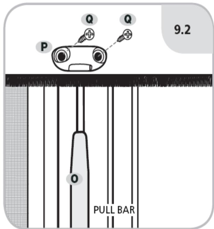
**SURFACE MOUNT INSTALLATIONS:** The Retainer Cups are not used in a surface mount installation. Drill a hole in the header and bottom sill of the door frame on which the unit is surface mounted that is large enough to receive the pointed end of the Slide Bolts.
